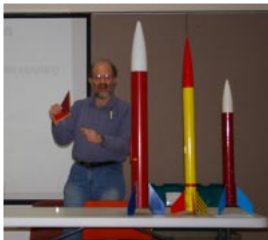
Bigger body tubes need bigger fins.
