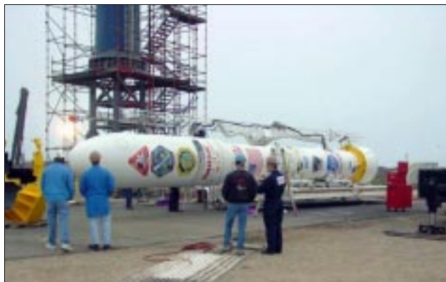
Failed Taurus T6 upper stages prior to stacking atop Castor 120 first stage. (NASA photo)
