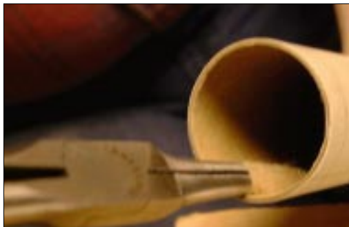
Using needle-nose pliers to modify the motor mount for standard motors.
