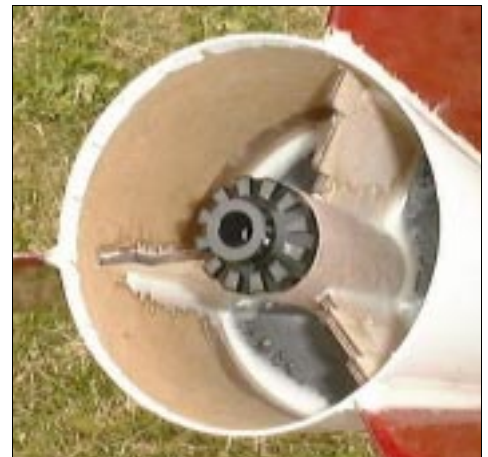
Attach fins before the rear centering ring so that internal fillets can be made.
